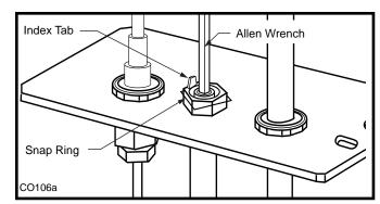
Fig. 60 Remove pilot orifice.
